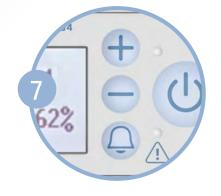
Set the flow setting to the flow rate prescribed by your clinical professional. The flow setting can be changed by pressing the circular flow setting buttons that are marked with "+" and "-" symbols. Position the nasal cannula on your face and breathe normally through your nose.
